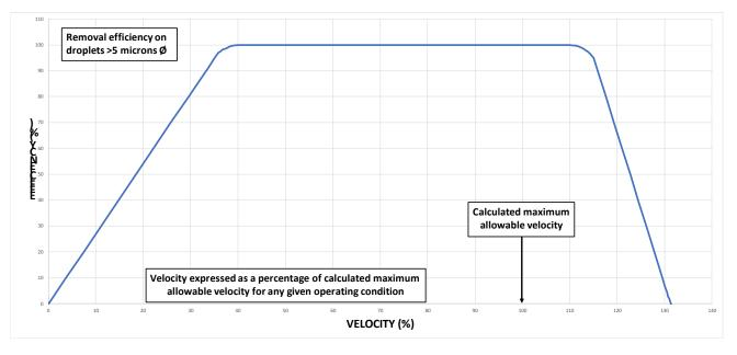
Fig. 5 Range of a Demister's Efficient Flow Conditions
