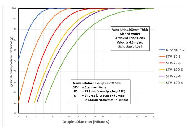
Fig. 4 Graph of Vane Pack Efficiencies
