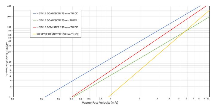
Fig. 7 Some Meshpad Demister Pressure Losses
